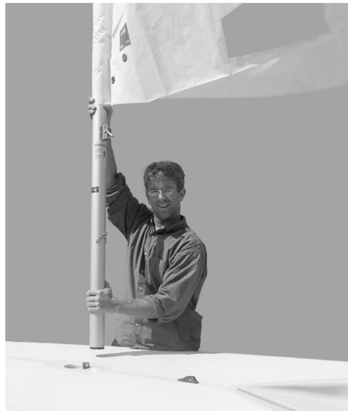
Figure D: Stepping the Mast
